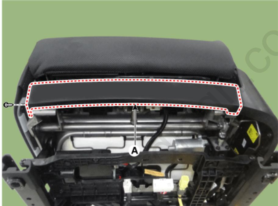
2. Remove the front seat outer shield cover (A) by using a remover.
